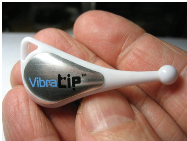
Figure 1. VibraTip®: a new device using standardised vibration for detection of peripheral neuropathy
